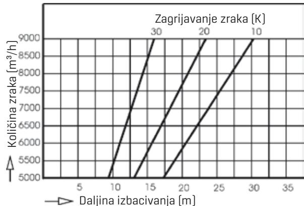
Primjer: LH 100 s ispušnom rebrenicom;  $\Delta t_i = t_{L\text{eff}} - t_{\text{prostora}} = 20 \text{ K}$ ; količina zraka = 7 300 m<sup>3</sup>/h
