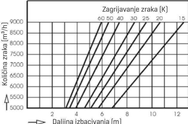
Primjer: LH 100 s ispušnom rebrenicom;  $\Delta t_L = t_{L\text{eff}} - t_{\text{prostora}} = 10 \text{ K}$ ; količina zraka = 7750 m<sup>3</sup>/h
